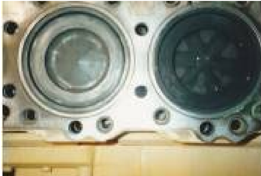
Figure 11 – Caterpillar 3412 Pistons after 14,000 operating hours using FPC
